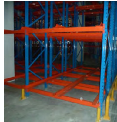
High Density Double Deep Pallet Racking
