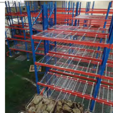
Racking with GI Wire Mesh Deck
