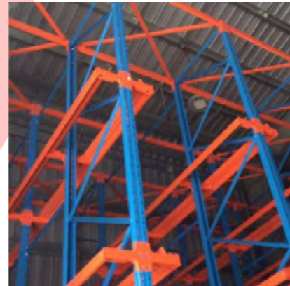
Drive In Pallet Racking
